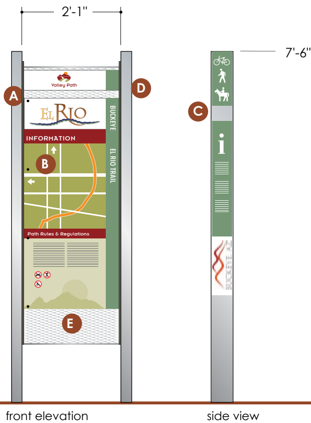
Valley Path standard trail kiosk modified for El Rio
